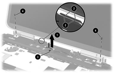
Removing the Display Assembly Screws
